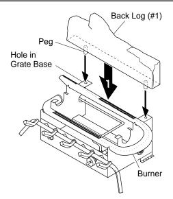
Figure 17 - Installing Back Log (#1)
